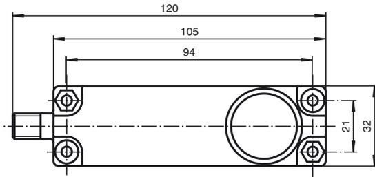
Bore hole and countersinking for screws/hexagon M4
