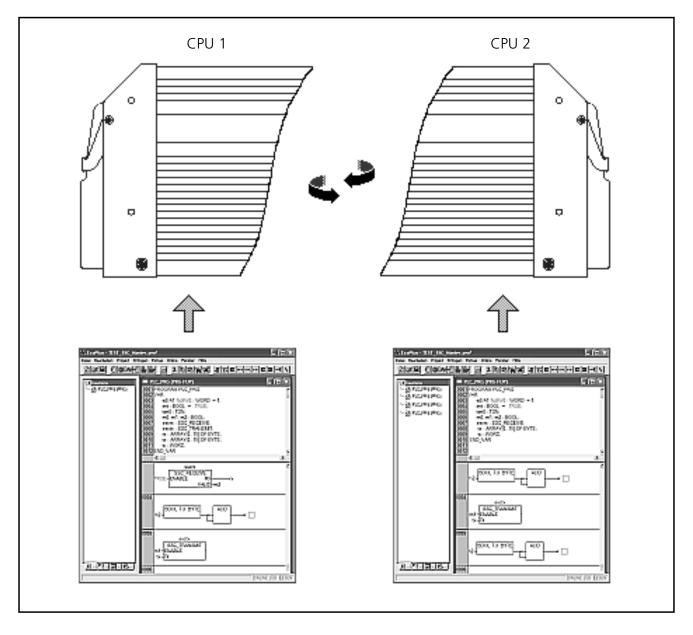
The 2 control units are treated by the programmer as 2 separate controllers. An IEC program is loaded into each control unit. The programs work in parallel and asynchronously.
