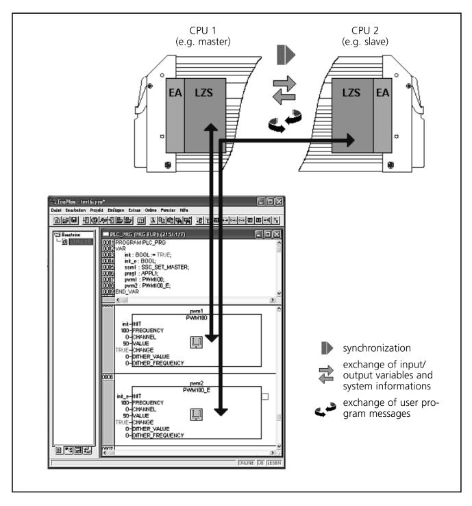
The 2 control units are treated by the programmer as one controller. The IEC program is processed in sequence, i.e. without parallelism.
