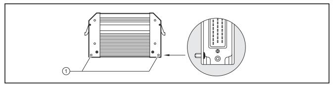
1: Drill holes for ground connection
