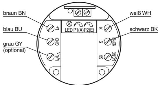
The terminals  $I_A/U_A$  (analog output) and SX (2<sup>nd</sup> switching output) are not needed for programming.
