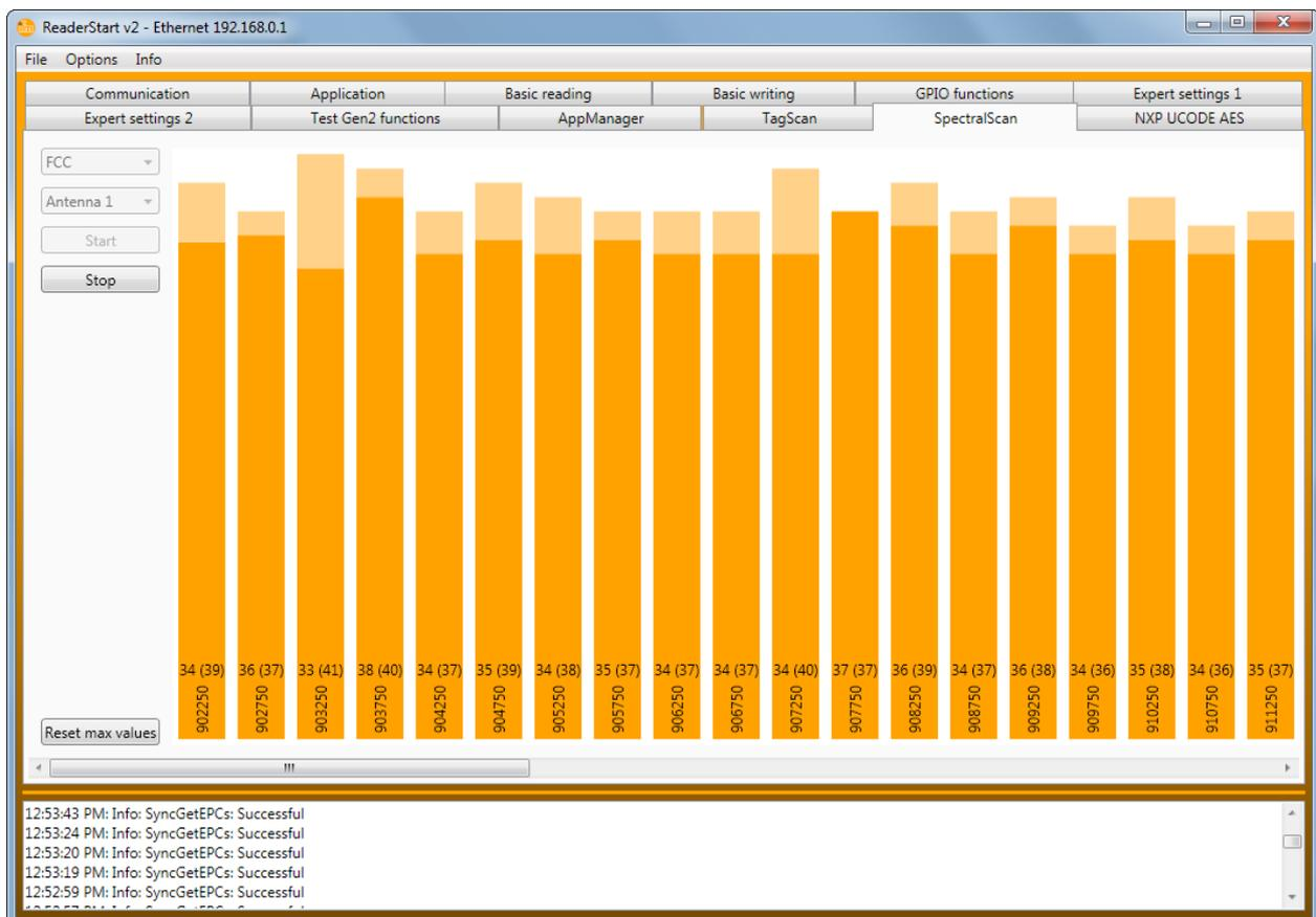
The mode "Dense Reader" and the free frequency selection permit trouble-free operation in spite of the neighbouring jammer. In the screenshot you can see that the ifm RFID reader uses channel 4. Alternatively channel 7, 10 or 13 would be possible. After 4 seconds the ifm RFID reader changes the channel.
