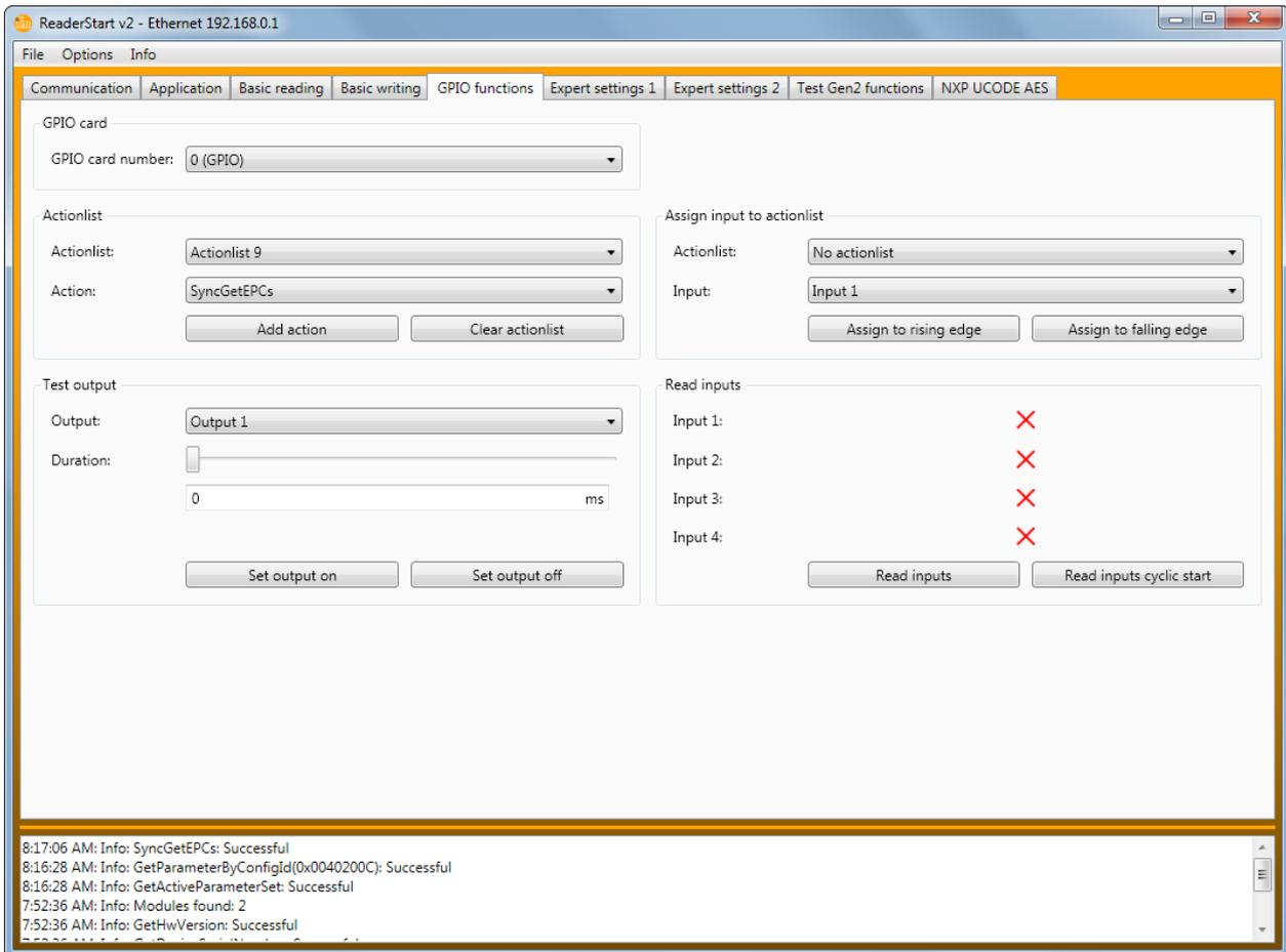
With "Add action" the commands are written to the selected action list in chronological order. Each added command is acknowledged in the system banner with the message "GPIOAddActionToActionlist(9): Successful". The number in brackets indicates the number of the selected action list ("9" in the message).
