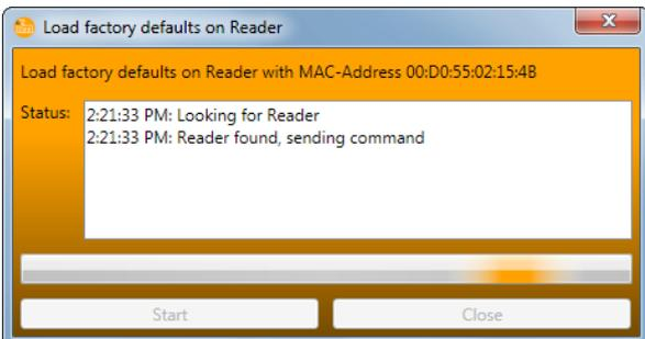
The reader was reset and can be accessed via the IP address 192.168.0.1.
