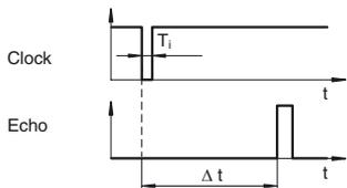
We recommend the usage of a npn-transistor to trigger the sensors clock input. The sensors clock input is connected to the +5 V potential internally by means of a pull up resistor.
