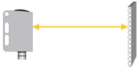
***Teach for 11% sensor sensitivity (highly transparent bottles and foils with thickness > 20µm)***
