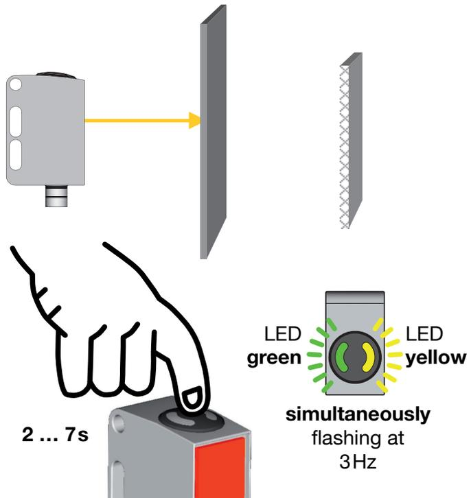
**Adjusting the switching behavior of the switching output – light/dark switching**
