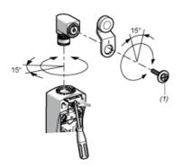
(1) Tightening torque (Min: 1) (Max: 1.5)
