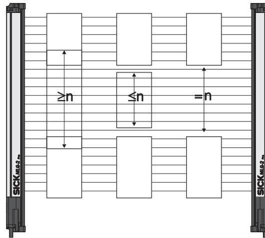
Figure 101: Hole detection/hole size
