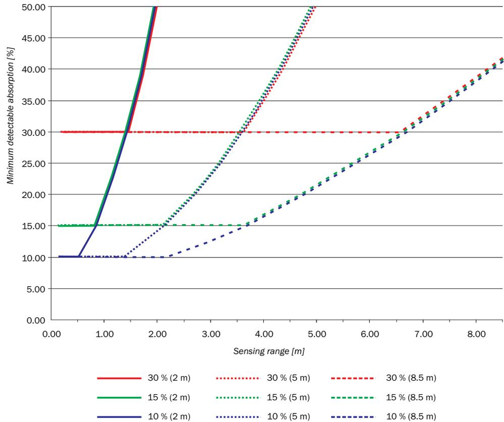
Figure 146: Minimum detectable absorption required for devices with 2 m, 5 m and 8.5 m sensing range
