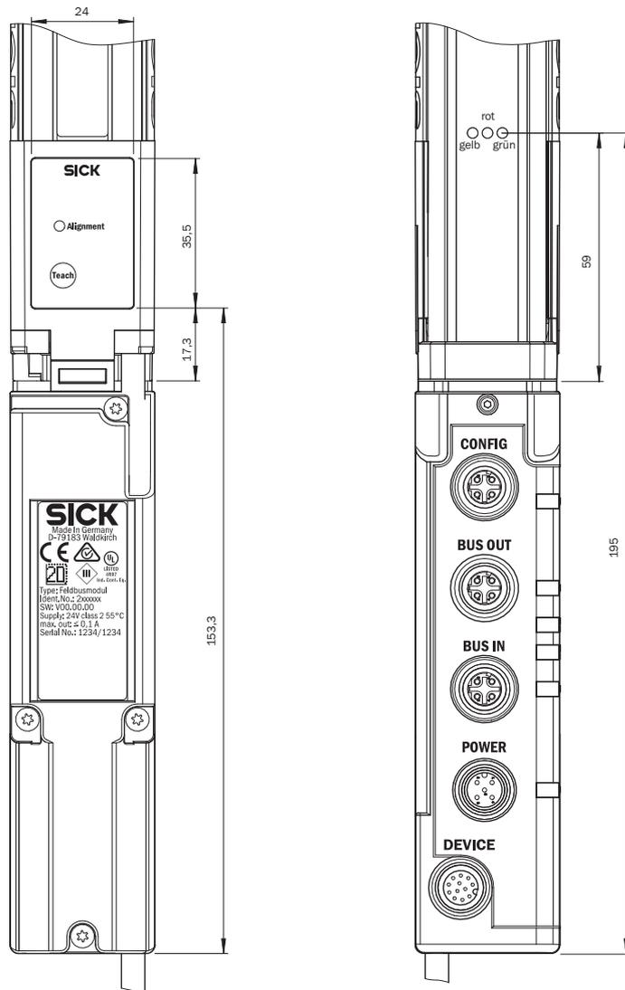
Figure 148: Dimensional drawing 1 MLG-2 fieldbus module
