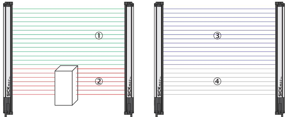
Figure 123: Example of the blanking of blocked beams
