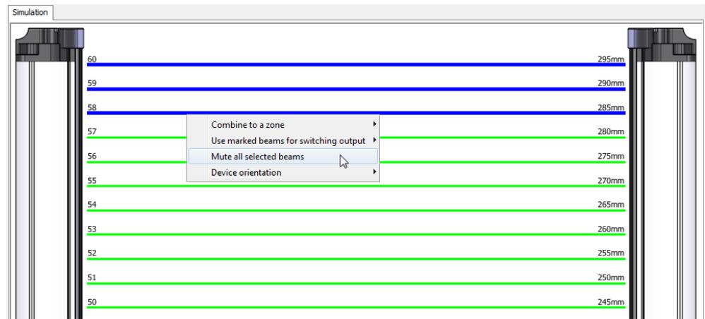
Figure 82: Blanking beams
