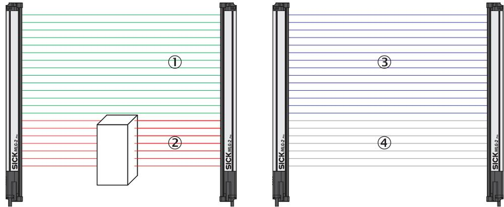
Figure 68: Example of the blanking of blocked beams
