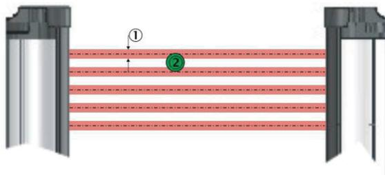
Figure 16: Minimum detectable object size with high measurement accuracy
