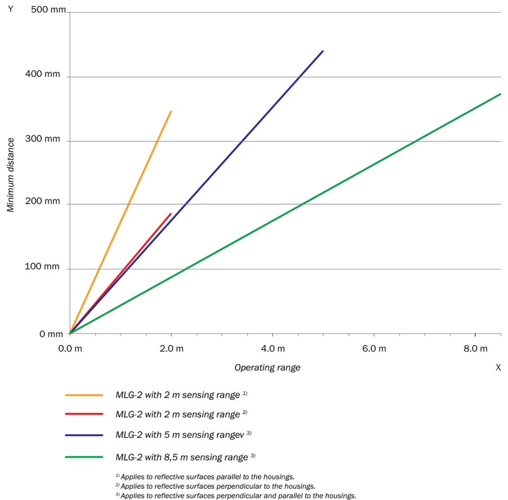
Figure 32: Graph, minimum distance from reflective surfaces
