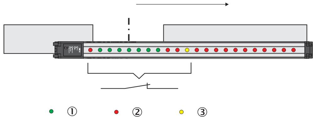
Figure 112: Classification of the hole position – smaller than or equal to hole center
