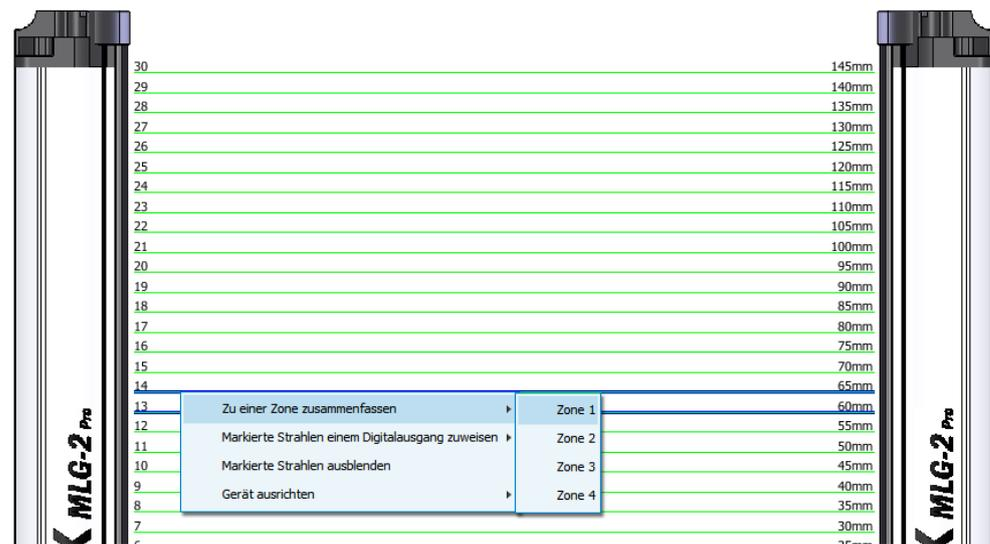
Figure 78: Combining beams into zones
