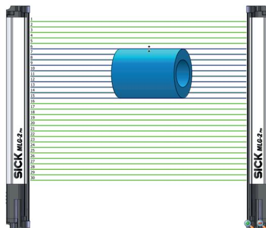
Figure 106: Setting the outside dimension with the mouse
