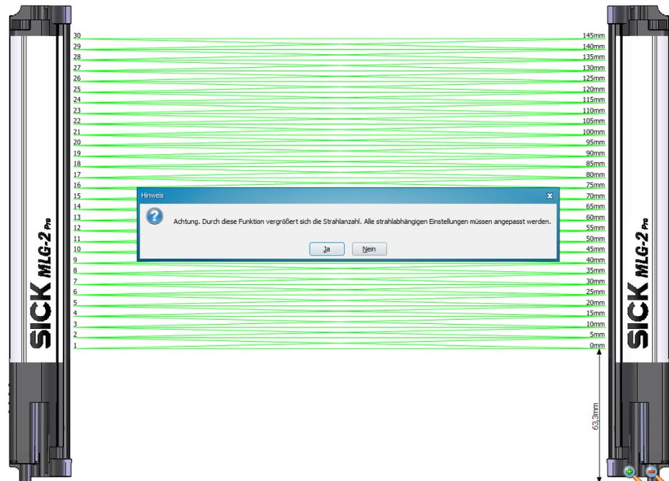
Figure 131: SOPAS ET, beam window – “Cross beam measuring” display
