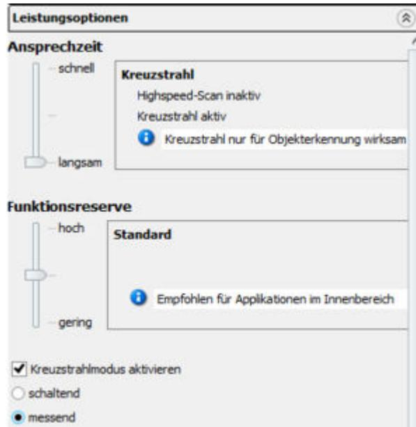
Figure 130: SOPAS ET – Activating cross beam measuring mode
