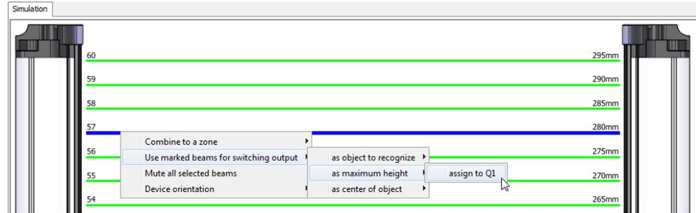
Figure 80: Using beams for height classification
