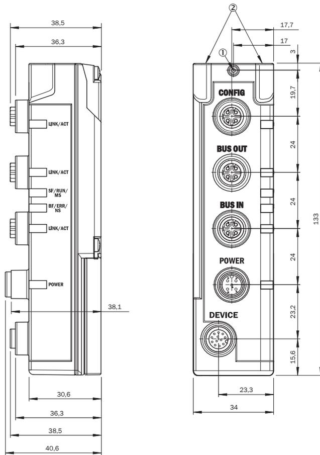
Figure 149: Dimensional drawing 2 MLG-2 fieldbus module
