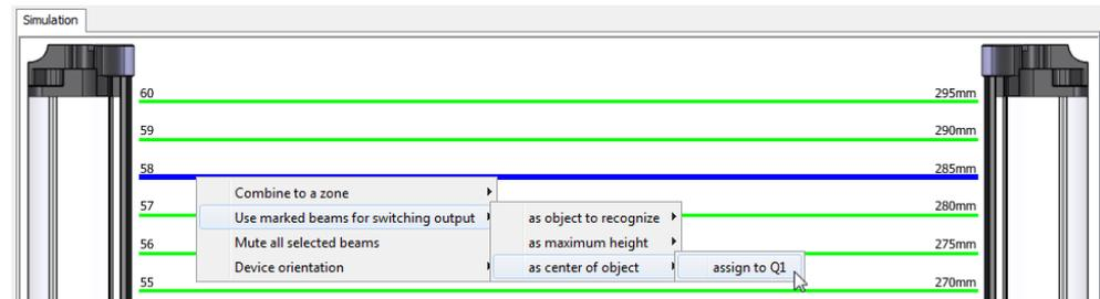
Figure 81: Using beams to classify the object position
