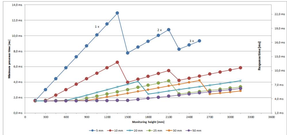
Figure 145: Response time and minimum presence time up to 8.5 m sensing range
