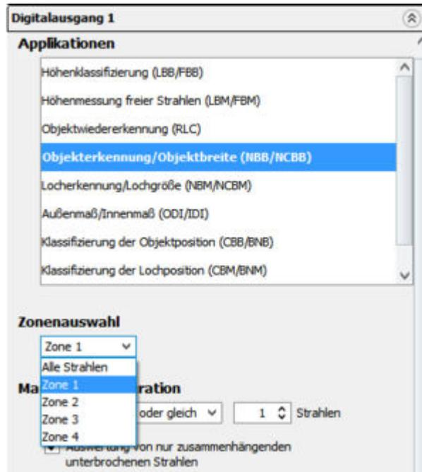
Figure 118: SOPAS ET – Assigning an application and zone to an output
