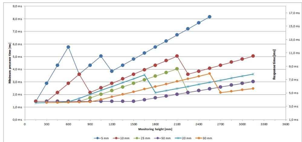
Figure 144: Response time and minimum presence time up to 3.5 m sensing range
