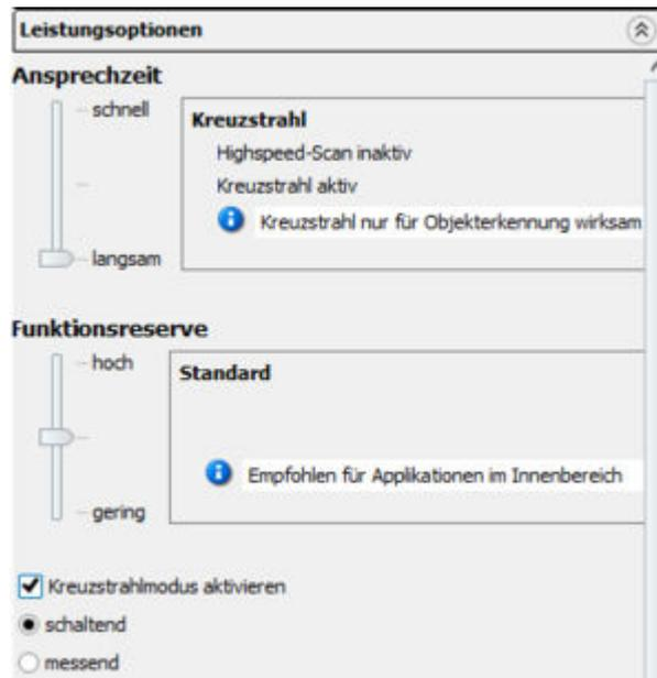
Figure 129: SOPAS ET – Activating cross beam switching mode
