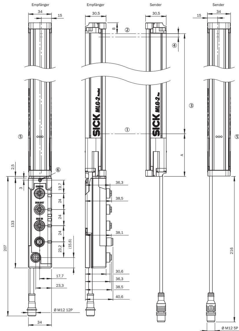
Figure 147: Dimensional drawing MLG-2 ProNet (mm)
