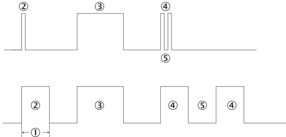
Figure 115: Examples of the effect of a configured minimum pulse width
