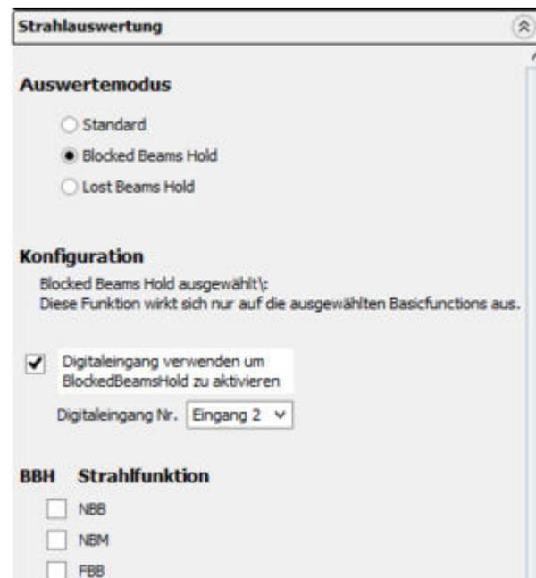
Figure 132: SOPAS ET – “Blocked Beams Hold (BBH)” function
