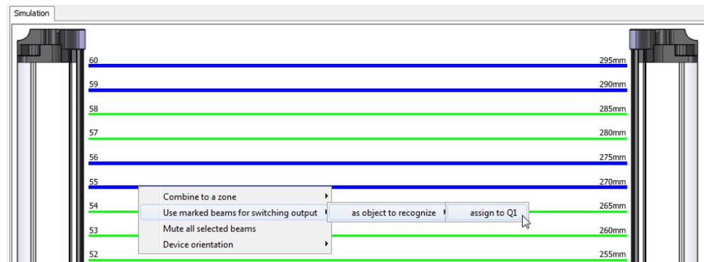
Figure 79: Using beams for object recognition
