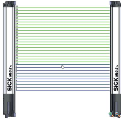
Figure 99: Setting the object size with the mouse
