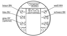
The terminals  $I_A/U_A$  (analog output) and SX (2<sup>na</sup> switching output) are not needed for programming.
