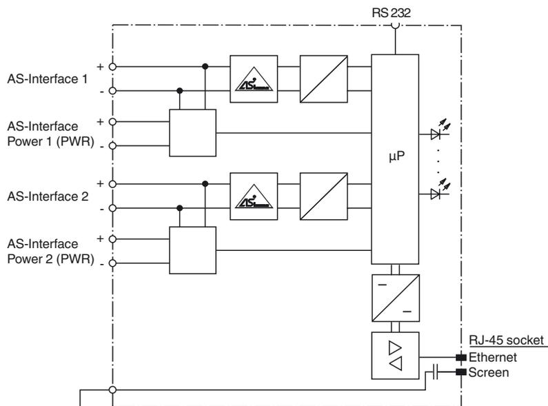
AS-Interface circuit 1 and 2 are supplied from different power supplies. At the cable for power supply no slaves or repeaters may be attached. At the cable for AS-Interface circuit no power supplies or further masters may be attached.
