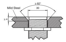
Sensor face is flush with mounting surface.
