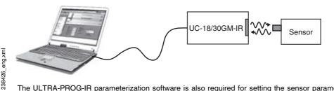
The ULTRA-PROG-IR parameterization software is also required for setting the sensor parameters. The ULTRA-PROG-IR software can be downloaded for free from the www.pepperl-fuchs.com website. The software allows all open parameters to be set, including:
