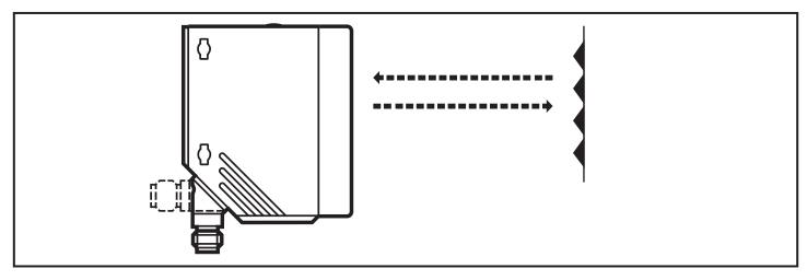
Place prismatic reflector or reflective tape behind the object to be detected. Align the photocell and fasten it to a mounting bracket.
