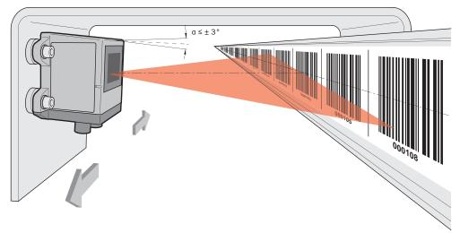
Figure 12: Vertical alignment
