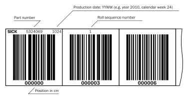
Figure 20: Bar code tape, height 30/40/60/100 mm
