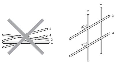
Figure 14: Cross cables at right angles
