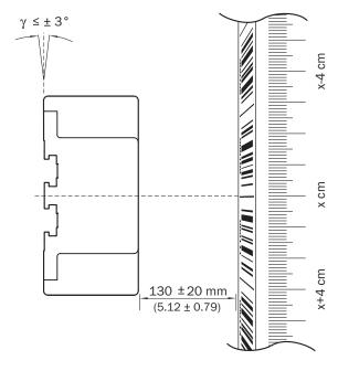
Figure 11: Mounting distances OLM100-xx5x
