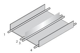
Figure 16: Alternative laying - Separate cables with metallic separators
