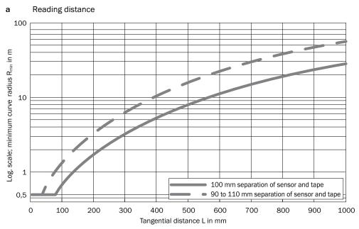
Figure 8: Minimum curve radius  $R_{min}$  dependent upon the tangential distance L
