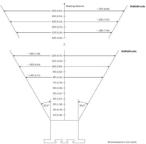
Figure 13: Field of view of the OLM100
