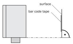
Figure 6: Vertical mounting of the bar code tape
