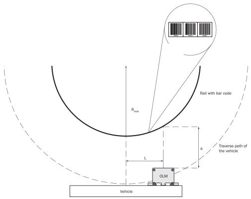
Figure 7: Tangential distance L for curve travel
