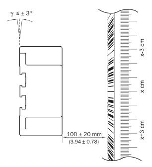
Figure 10: Mounting distances OLM100-xx0x
