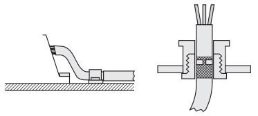
Figure 18: Shield connection in plastic housings
