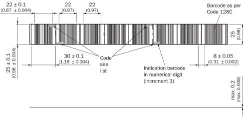
Figure 21: Bar code tape, 25 mm height
