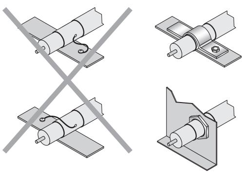
Figure 17: Make an extensive and low-impedance ground connection of the cable shield in the control cabinet.
