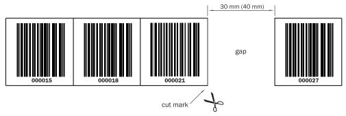
Figure 5: Gap in the separated bar code tape
