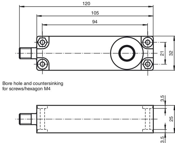
Bore hole and countersinking for screws/hexagon M4
