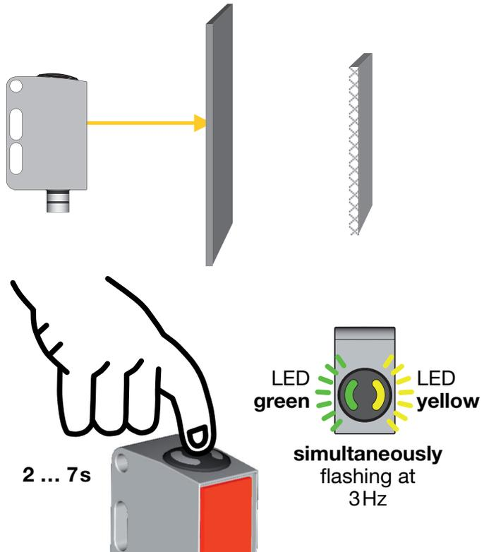
**Adjusting the switching behavior of the switching output – light/dark switching**
