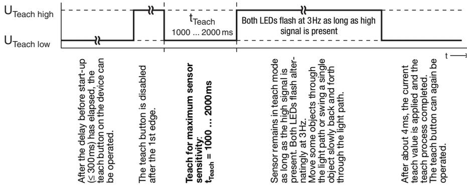
In the event of a teach error (e.g. no teach object or a teach object which is too small or too transparent is moved through the light path), the two LEDs flash at the same rate. Check the system, repeat the teach process, if necessary use a larger or less transparent teach object.
