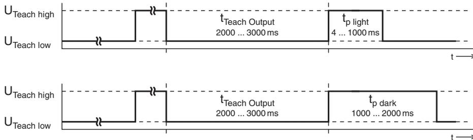
After the delay before start-up (<= 300ms) has elapsed, the teach button on the device can be operated.
