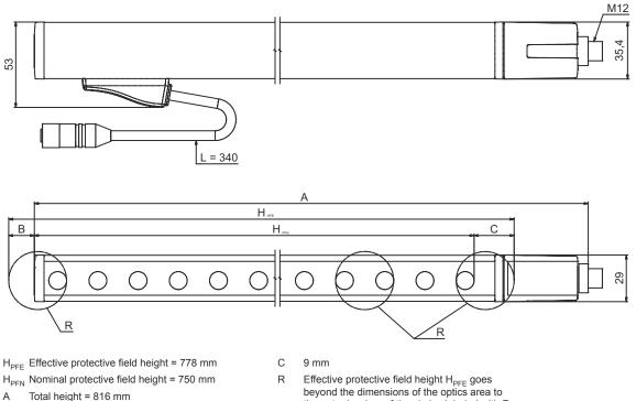
В 19 mm Effective protective field height  $\rm H_{\rm PFE}$  goes beyond the dimensions of the optics area to the outer borders of the circles labeled with R.
