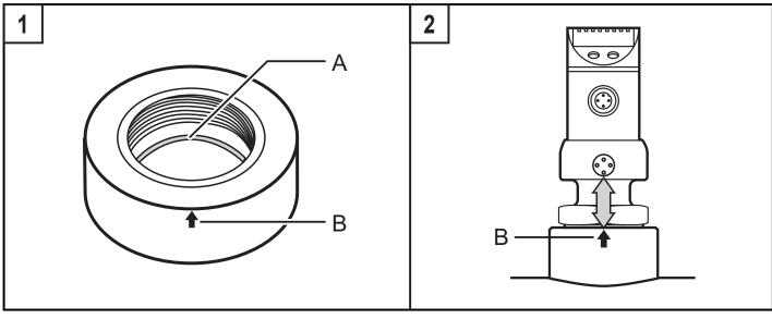
A: Groove for the O-ring (E30072 only); B: Marking for alignment
