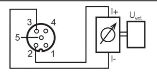
Connection of a 3-wire sensor without own supply
