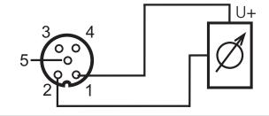
Wiring of a 2-wire sensor with electrically isolated and earth-free supply
