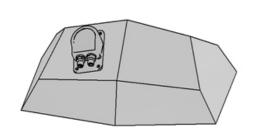
Inclination sensor installed at an angle in the coordinate system of the workpiece. The coordinate system of the sensor is transferred to the coordinate system of the workpiece by teaching the sensor when the workpiece is horizontally aligned.
