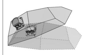
The raw data of the sensor is indicated in the coordinate system of the sensor.
