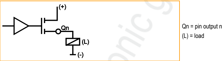
Basic circuit of output plus switching (BH) for positive output signal
