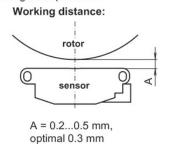
Use the distance band as s mounting tool for optimal gap (0.3 mm) between sensor and rotor.
