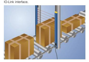
As these light curtains for measurement tasks are equipped with an integrated evaluation unit, external connection units are not needed. Objects are both rec-
