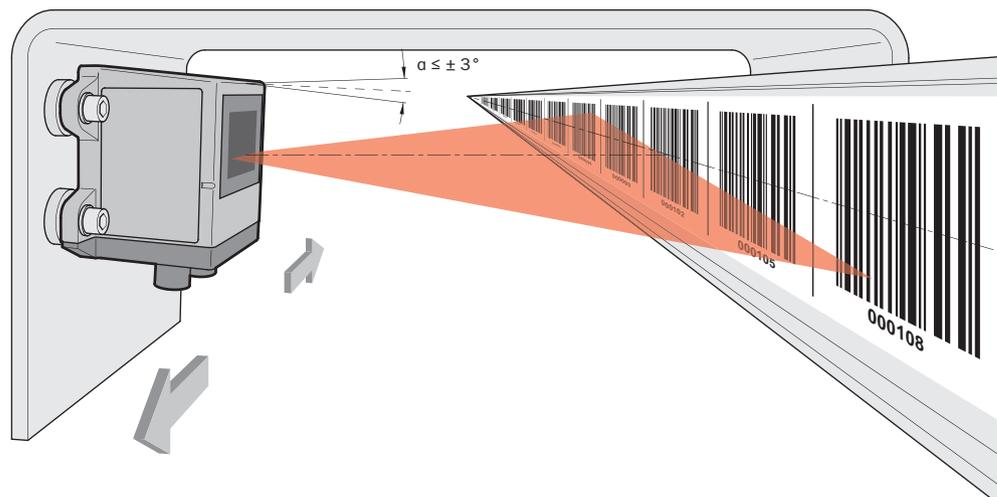
Figure 12: Vertical alignment
