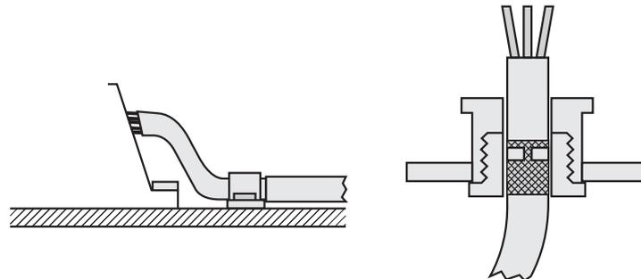
Figure 18: Shield connection in plastic housings
