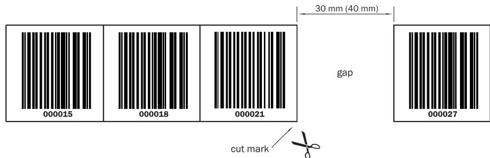
Figure 5: Gap in the separated bar code tape
