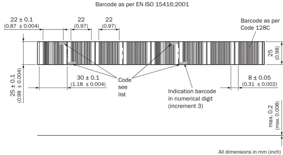
Figure 21: Bar code tape, 25 mm height
