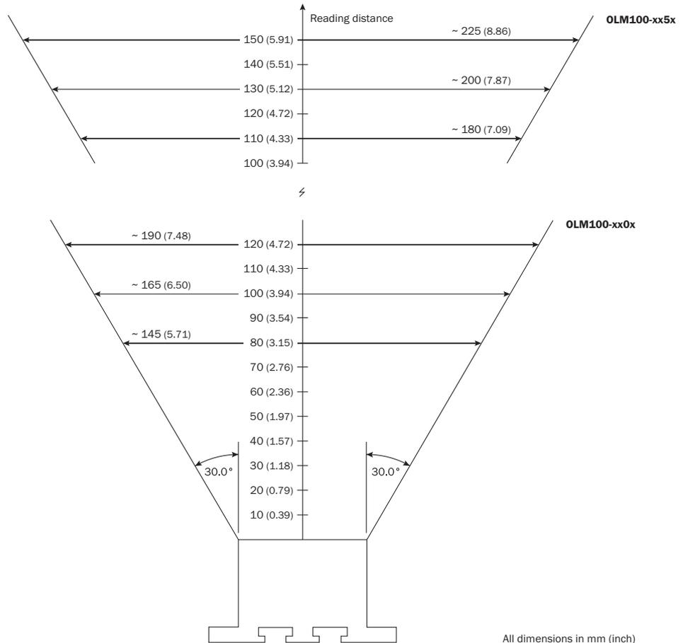
Figure 13: Field of view of the OLM100
