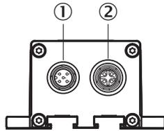
Figure 19: Position of the electrical connections
