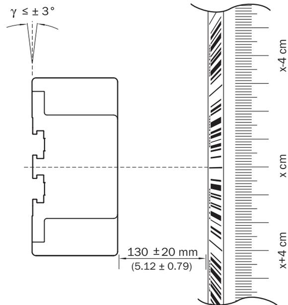
Figure 11: Mounting distances OLM100-xx5x
