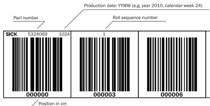
Figure 20: Bar code tape, height 30/40/60/100 mm
