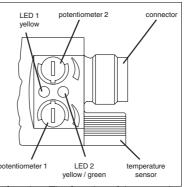
The potentiometer function described illustrates the default function. The function of the potentiometer can be altered using the ULTRA-PROG-IR software. As soon as a configuration has been changed, the potentiometer function selected using ULTRA-PROG-IR is activated.
