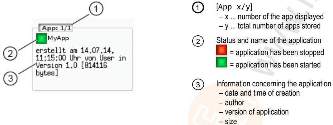
To control a single PLC application stored on the device:
