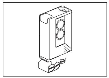
► Secure the mounting fixture with the screws supplied, then slide the unit into the slot of the fixture until the spring clicks home.
