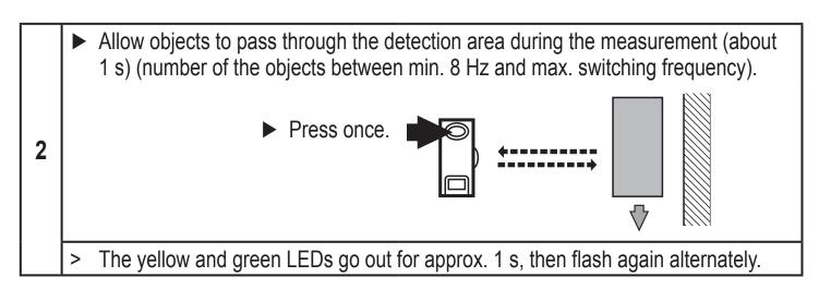
► Allow objects to pass through the detection area during the measurement (about 1 s) (number of the objects between min. 8 Hz and max. switching frequency).
