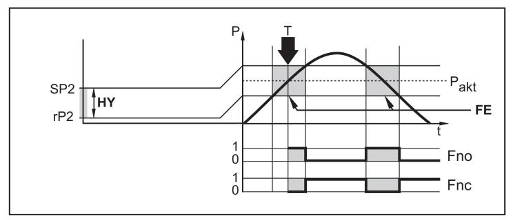
P = system pressure; Pakt = current system pressure; FE = window; T = time of teach
