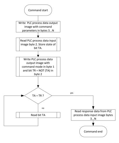
Note: It is allowed to setup the command mode and the command parameter in one PLC cycle, together with bit TR = NOT (TA), to activate the command.
