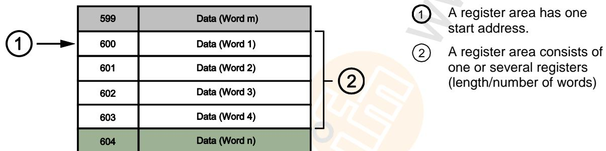
The following general rules apply for access to the Modbus registers:
