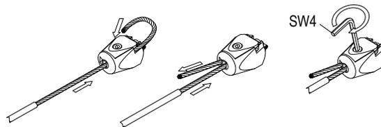
Figure 7. Install the Rope with Integral Turnbuckle
