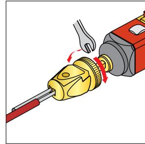
Figure 10. Applying tension to the rope (models RP-LS42F-..LE)
