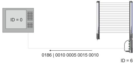
Figure 56: Example for process data
