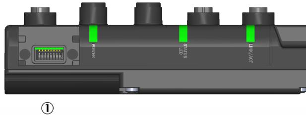
Figure 21: DIP switch on the fieldbus module
