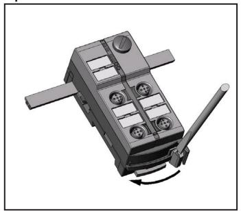
Open the unit using a tool as shown (e.g. screwdriver).
