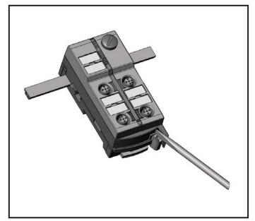
Take care in laying the AS-i flat cable, the flat cable should be laid straight for about 15 cm.
