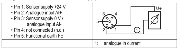
Wiring of a 2-wire sensor with electrically isolated and earth-free supply
