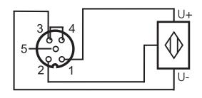
When connecting a 2-wire or 3-wire sensor without own supply there has to be an external link between pin 3 and pin 4.
