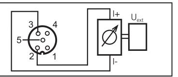
Wiring of a 3-wire sensor without own supply
