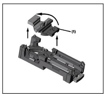
With the supplied lower part the flat cable can be aligned in three directions.
