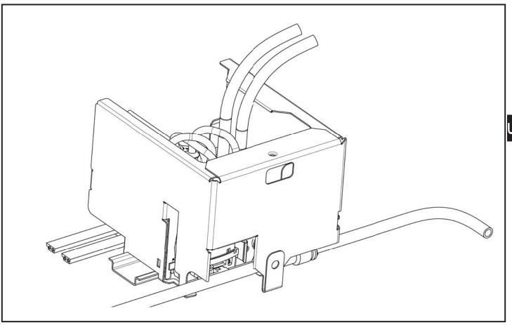
► Attach the cover, clip it into place and tighten the screw
