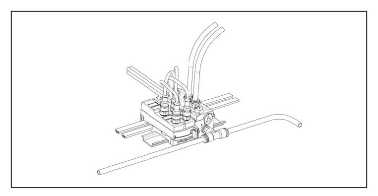
► Attach the frame to the DIN rail and clip it into place
