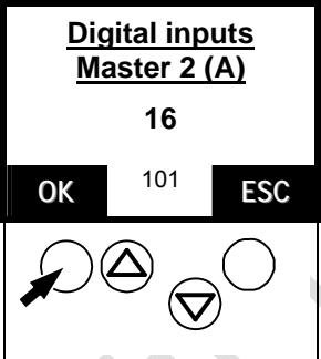
> Indicates that the fieldbus module 3 (digital input master 2(A)) with a length of 16 bytes is activated.
