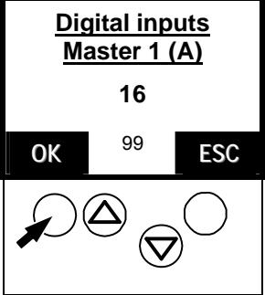
> Indicates that the fieldbus module 1 (digital input master 1(A)) with a length of 16 bytes is activated.
