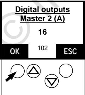
> Indicates that the fieldbus module 4 (digital output master 2 (A)) with a length of 16 bytes is activated.
