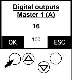
> Indicates that the fieldbus module 2 (digital output master 1 (A)) with a length of 16 bytes is activated.
