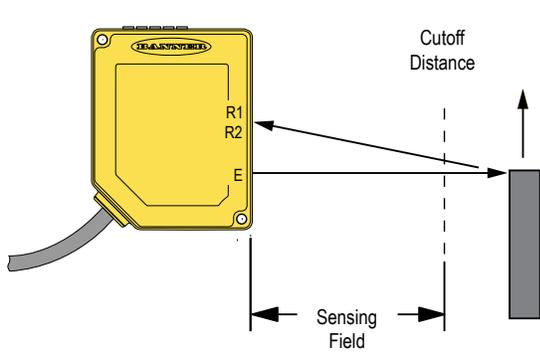
A reflective background object in this position or moving across the sensor face in this axis and direction may cause a false sensor response.
