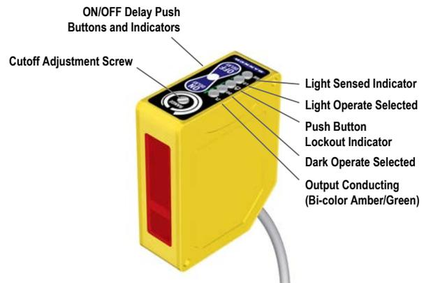
The indicators, above right, also function as a 5-segment light bar during delay selection modes
