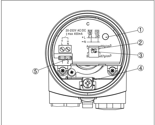
Fig. 9: Electronics and connection compartment, single chamber housing
