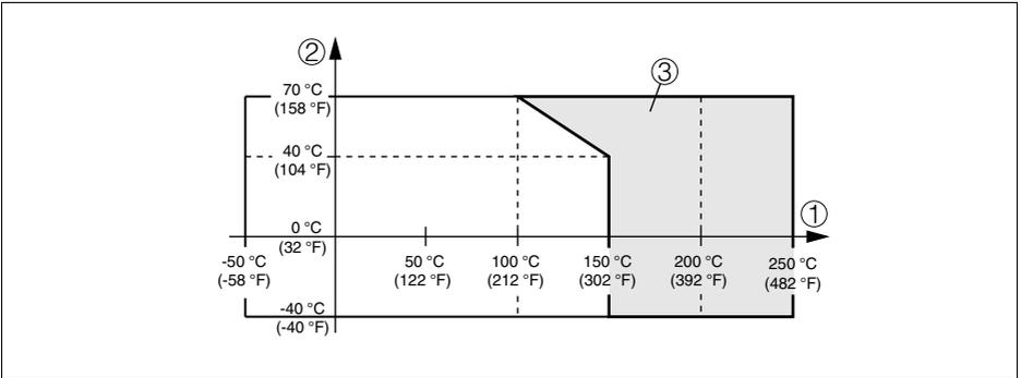
Fig. 28: Ambient temperature - Process temperature
