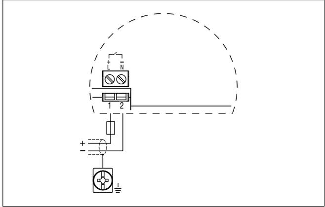
Fig. 10: Wiring plan, single chamber housing
