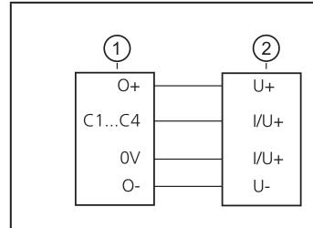
An actuator with separate supply is connected to the external 24 V via the terminals O+ and O-. The signal can be taken from the terminals C1/2 and COM1/2.
