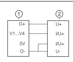
An actuator with separate supply is connected to the external 24 V via the terminals O+ and O-. The signal can be taken from the terminals V1/2 and COM1/2.
