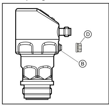
➤ Screw the filter cover with integrated pressure compensation diaphragm (D) onto the base (B) and tighten using a spanner, across flats 11\*).
