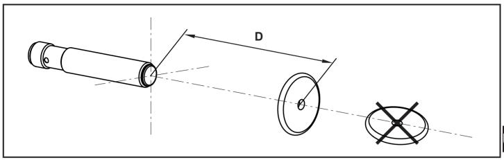
► Align the ID tag on the antenna central axis.
