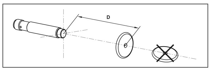
► Align the ID tag on the antenna central axis.
