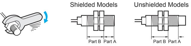
**Note:** 1. The allowable tightening strength depends on the distance from the edge of the head, as shown in the following table. (A is the distance from the edge of the head. B includes the nut on the head side. If the edge of the nut is in part A, the tightening torque for part A applies instead.)
