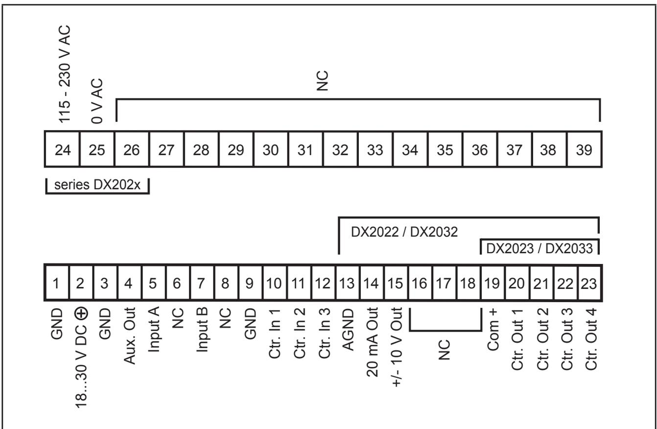
Connections on the rear of the housing
