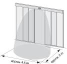
Mounting height 2200 mm / tilt angle 30° Antenna position:
