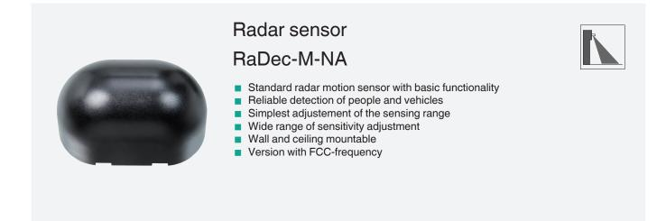
FCC-approved standard radar motion sensor with basic functionality. 2 m x 4.5 m detection range. Max 4 m mounting height. Black housing. Relay contact output. Cable connection.
