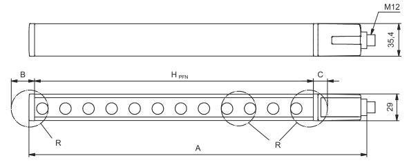
$H_{\mathrm{PFE}}$  Effective protective field height = 2340 mm  $H_{\mathrm{PFN}}$  Nominal protective field height = 2250 mm
