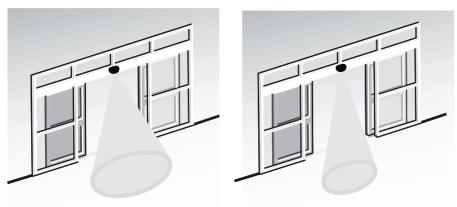
The size of the detection area can be changed using the potentiometer.
