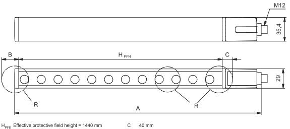
$H_{PFN}$  Nominal protective field height = 1350 mm
