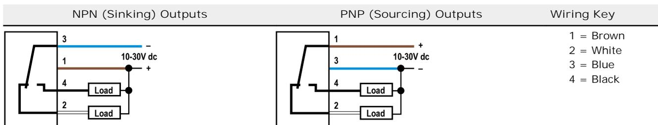
Cabled wiring diagrams are shown. Quick disconnect (QD) wiring diagrams are functionally identical.
