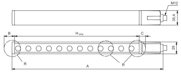
$H_{\mathrm{PFE}}$  Effective protective field height = 1840 mm  $H_{\mathrm{PFN}}$  Nominal protective field height = 1800 mm
