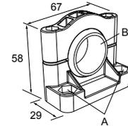
Hole center spacing: A=ø 50.8
